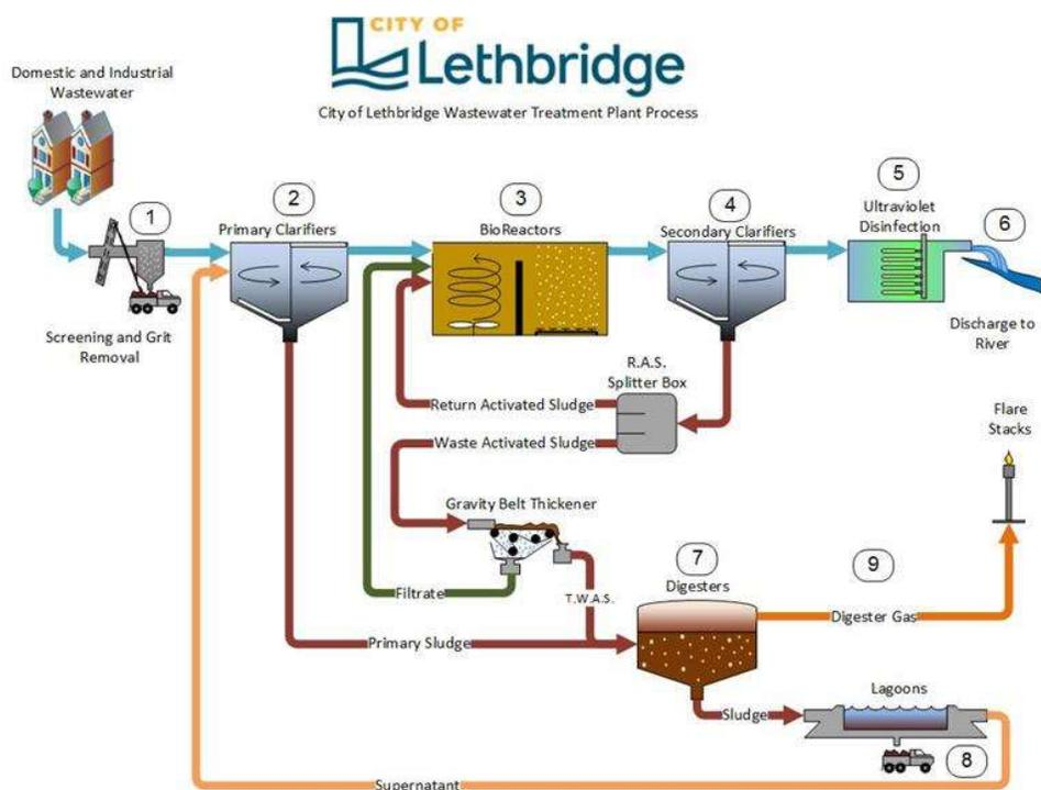
Figure 1. Process by which wastewater is treated in the City of Lethbridge's wastewater treatment plant (City of Lethbridge, 2022c).
